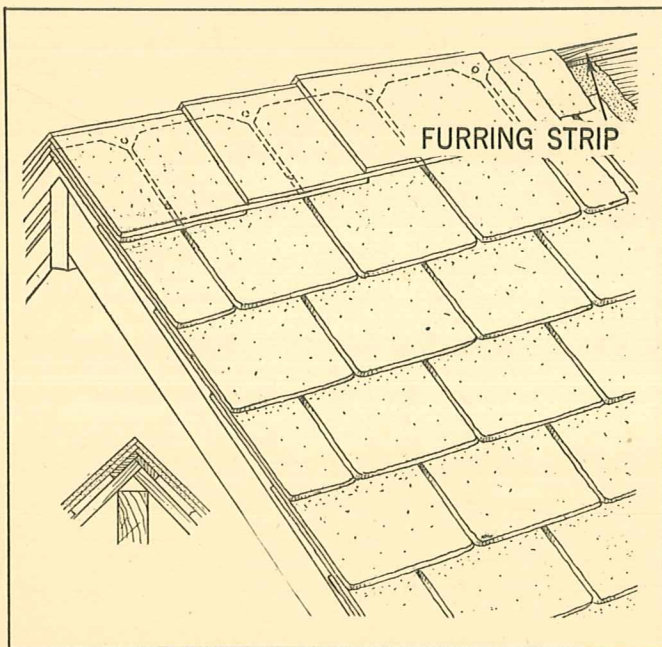
Figure 22—Boston Ridge construction
